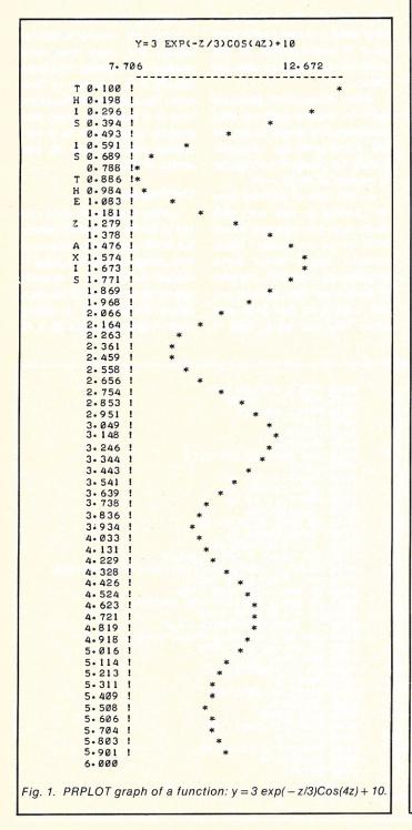
the equation for a sine wave that decays exponentially. We will plot it for z = 0 to z = 6.
